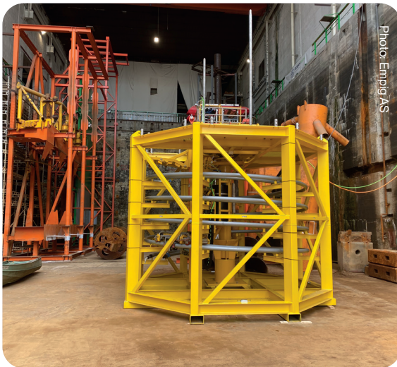
The picture shows the cooler in dry dock in Trondheim where the mechanical system was recently qualified in a shallow water test.
