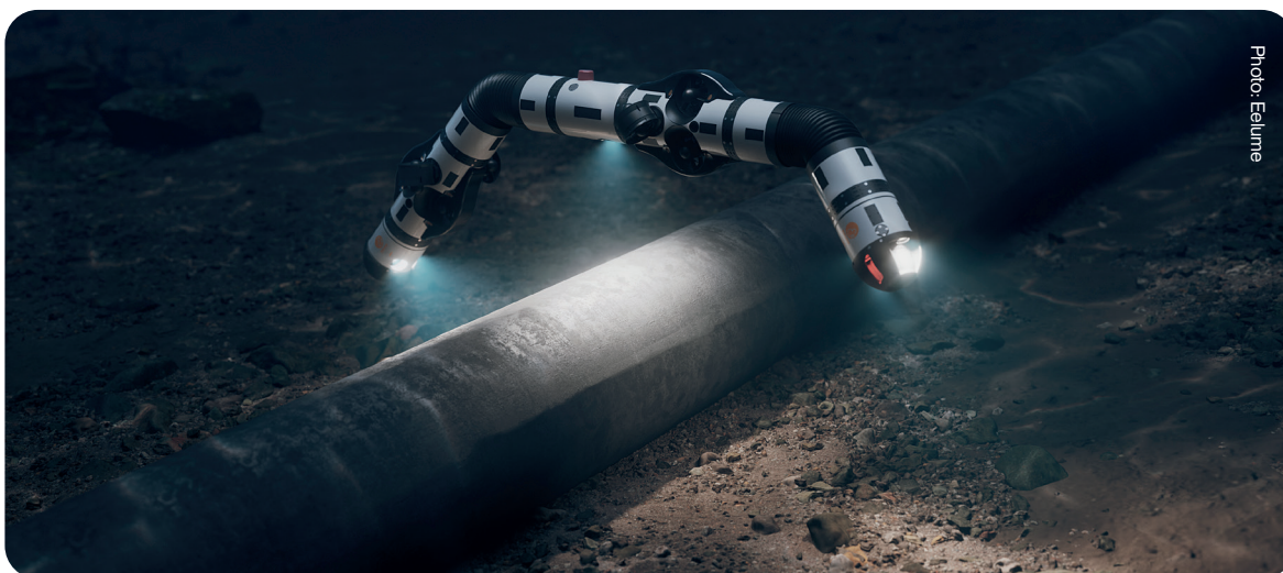
Eelume executes pipeline inspection on the seabed
