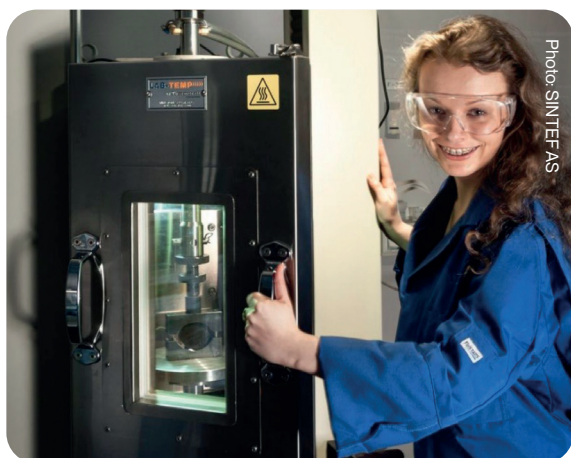
Mechanical testing in a load cell, to see if different rocks in the underground are weakened after exposure to hydrogen.
