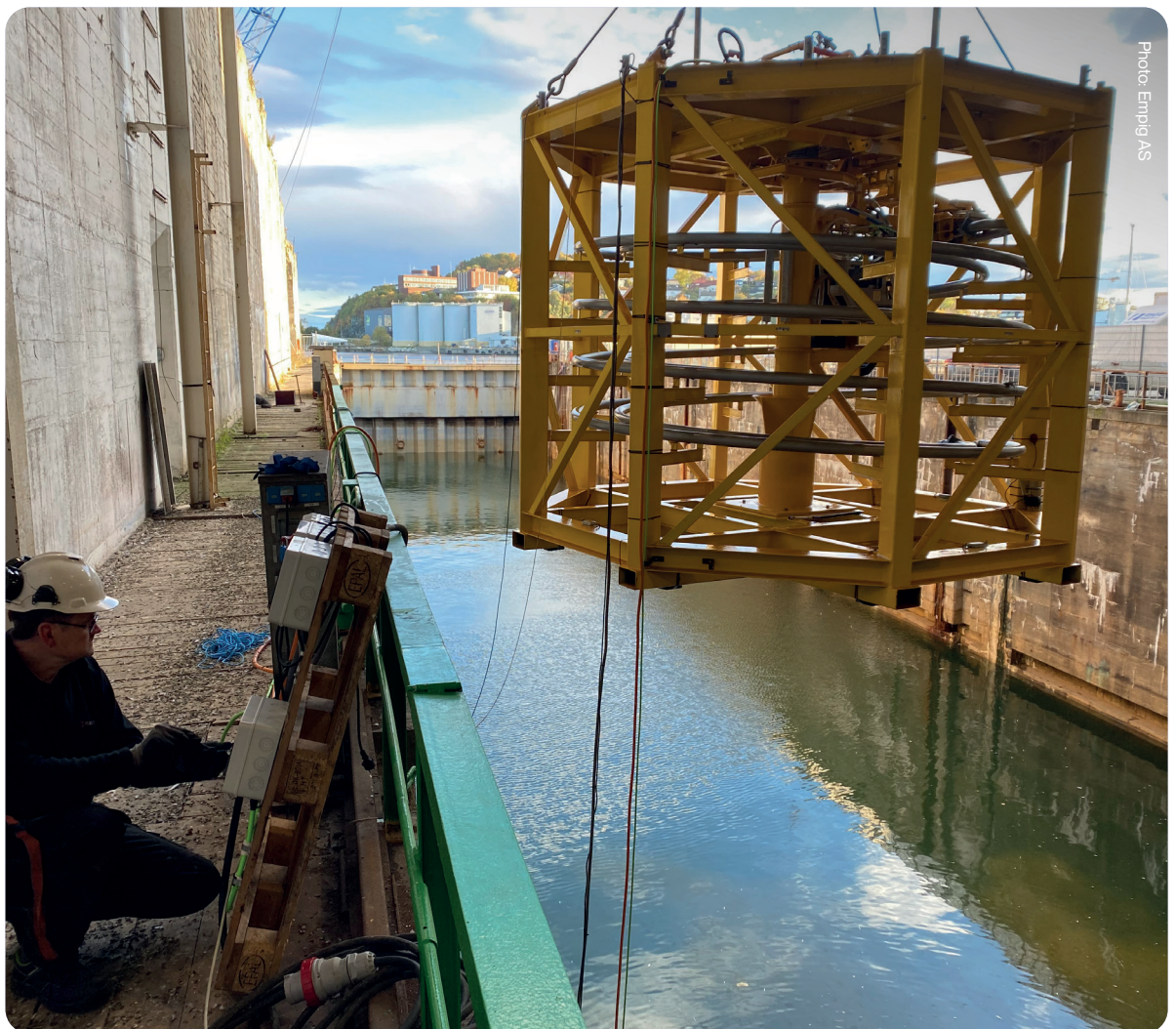
Mechanical shallow water TRL4 test of Empig's underwater cooler
