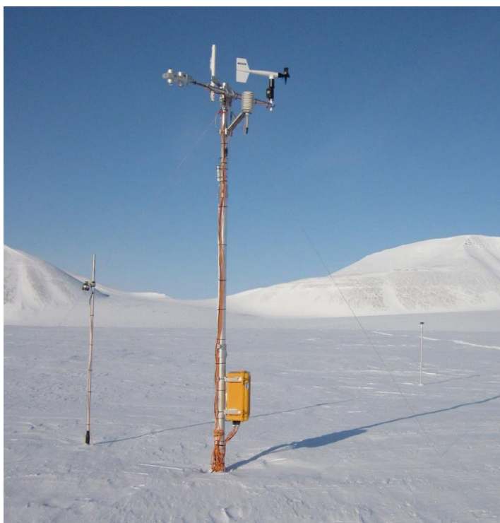
Figure: Photo of the Automatic weather station on Nordenskiöldbreen in April 2011. (Photo: A. Waxegard).
