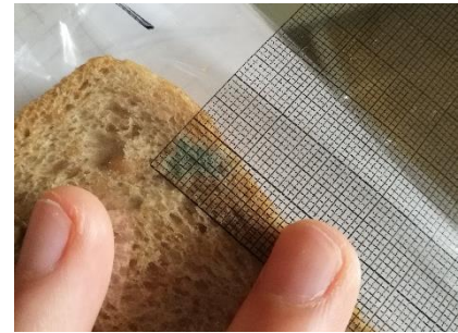
Figure 2 Usage of the gridded sheet to measure the moulded area.
