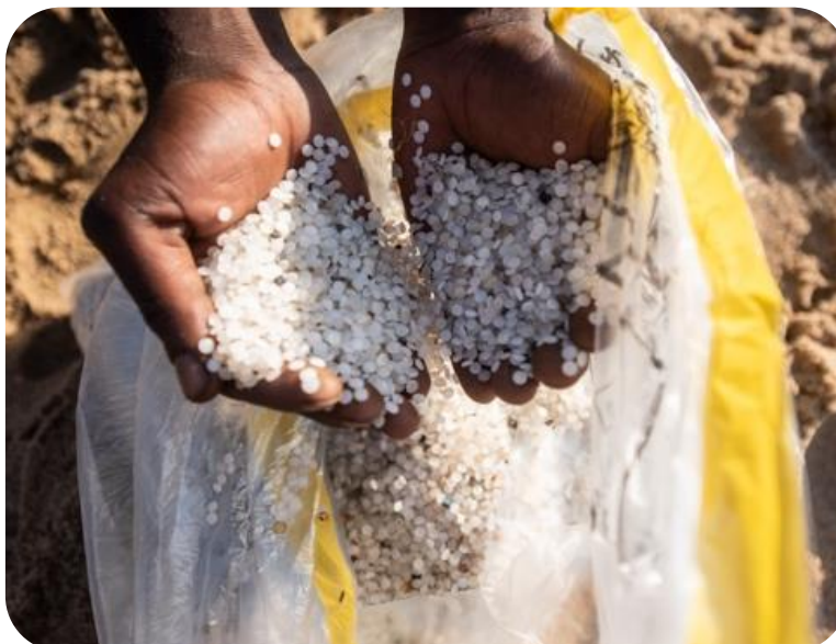
Pre-production microplastic pellets, also known as nurdles, collected during the research period. Photo: WildOceans
