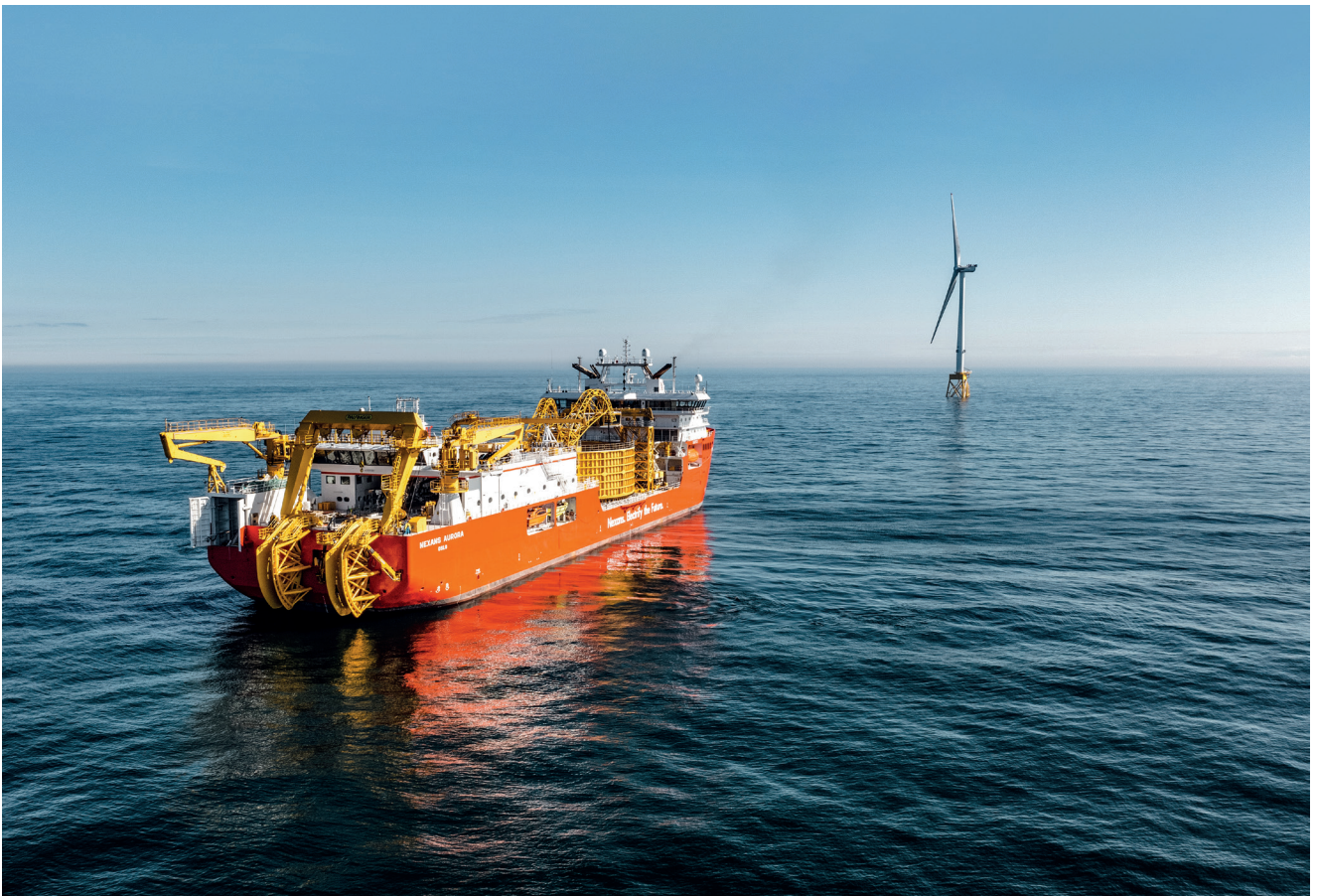
Cable installation vessel Nexans Aurora. Photo: Nexans
