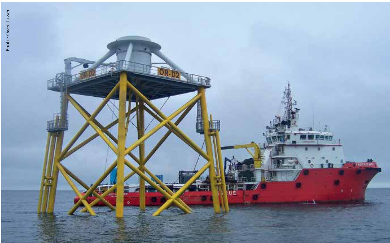
The foundation for an offshore wind turbine.
