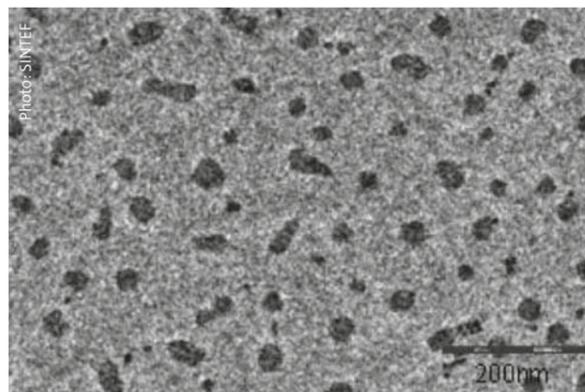
Silica capsules with particles averaging just 30 nm in size, as seen through a transmission electron microscope.
