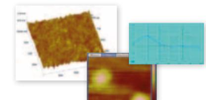
Atomic force microscope (AFM) image of nanosheets on a surface. The nanosheets are roughly 1 nm thick with a diameter of 20-30 nm.
