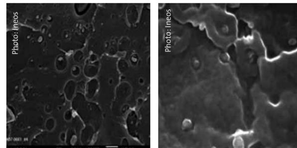
Electron microscope images of post-impact fracture surfaces of PVC foam. Left: Poor mechanical properties due to insufficient contact between nanoparticles and the foam material. Right: Good nanoparticle-to-foam contact results in vastly improved impact strength.
