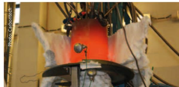
Pilot facility for production of carbon nanoparticles.
