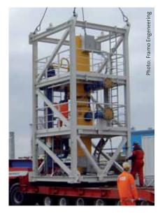
WET GAS COMPRESSOR: This compressor enable gas export either onshore, offshore or subsea.
