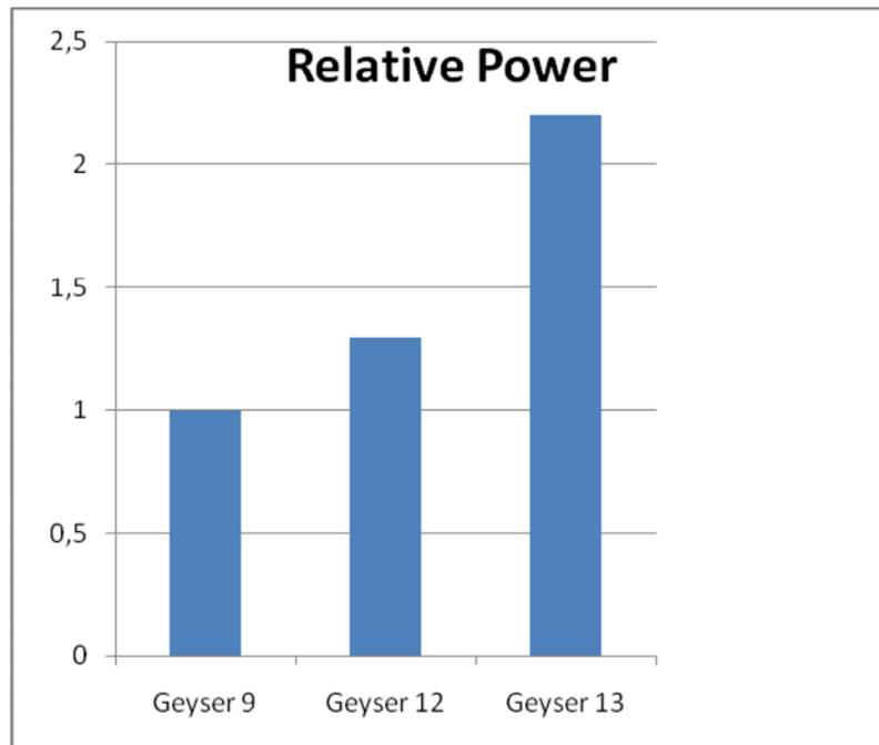
Figure 65 – The relative difference of the three heat settings
