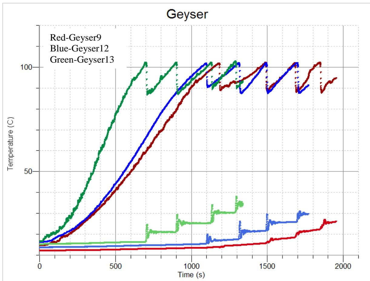
Figure 13 – A comparison of the geysers with different heating settings
