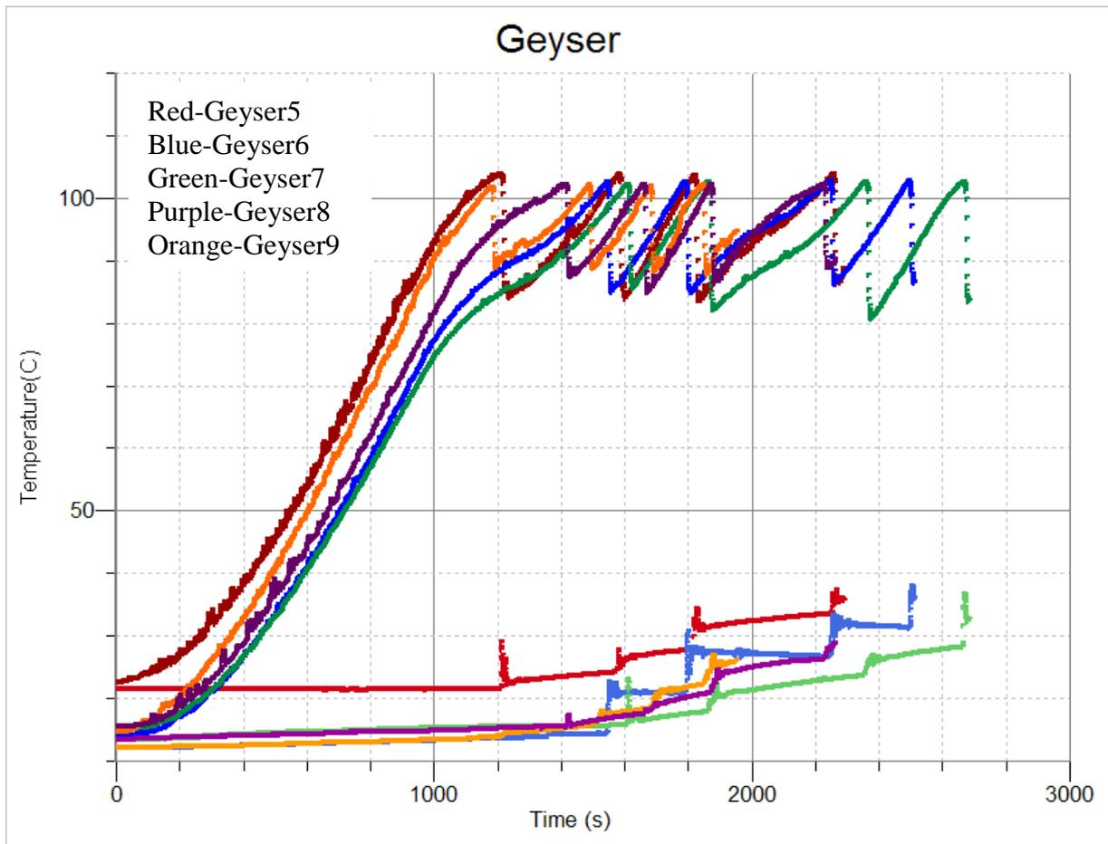
Figure 5 – The geysers with straight tubes and different heights
