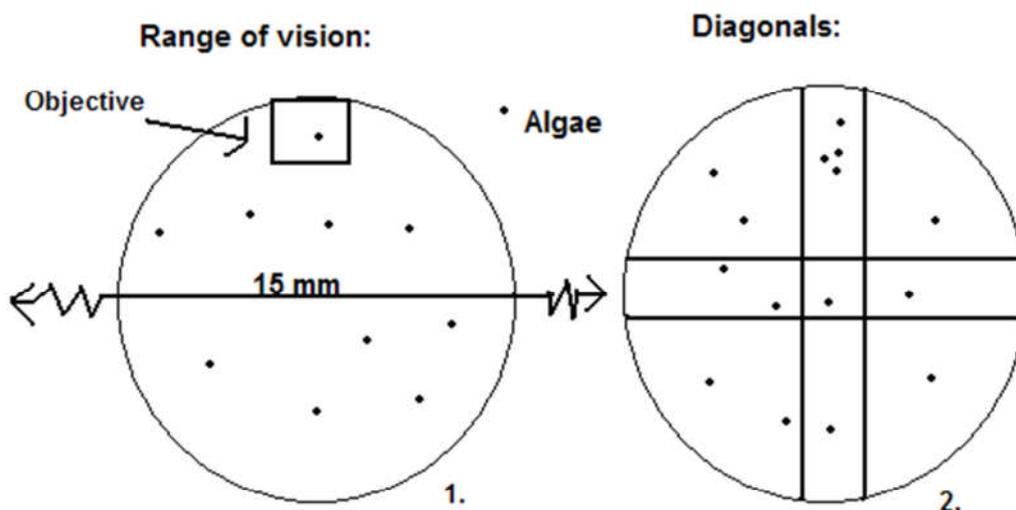
**Figure 2.3: 1.** Illustration of the range of vision and the width of chamber in the light microscope. **2.** Illustration of how the diagonals were counted either up and down, or from left to right and opposite
