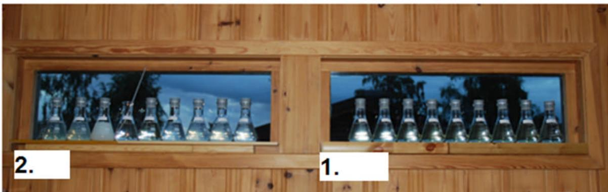
**Picture 2.2: The position of the flasks in relation to its surroundings.** The flasks are positioned away from the wall and above the window frame. The control groups were placed in the middle (photo: private)
