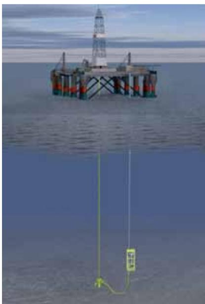
GOING DEEP: AGR has developed a method that make it possible to drill in deep water without pipe liners for reinforcement. Photo: AGR
