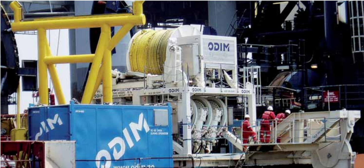
PROTECTION: ODIM's CTCU uses individually controlled sheaves which move at different speeds, protecting the fibre rope. Photo: ODIM
