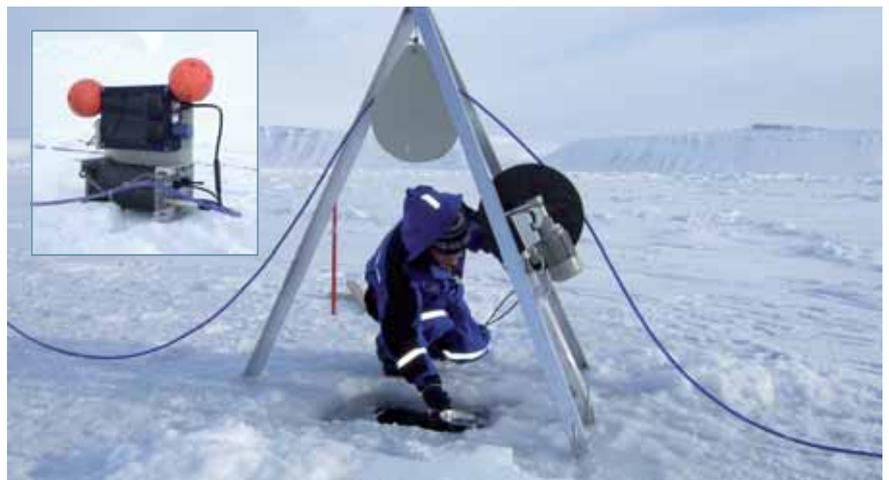
DOWN UNDER: Lowering the Echoscope through a hole in the ice. The insert shows Echoscope mounted on a frame with a data unit and cable for lowering into water. Photo: NERSC
